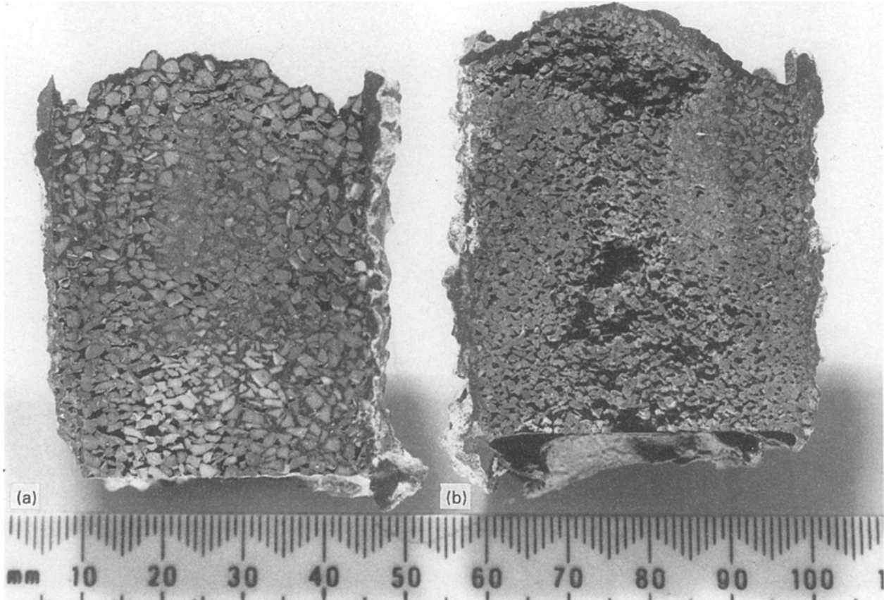
Figure 3 Cross-sections of the products with (a) T60A, and (b) T60B, by firing for 15 h at 1180 °C.
